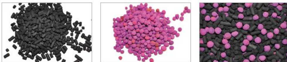
Figure 4: Activated carbon pellets, BAC granules, mixture of activated carbon & BAC
