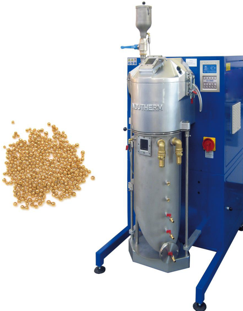
GU3000 with some customer specific options on granulation tank
