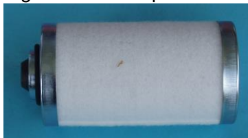
Figure 29: Oil separator filter of vacuum pump
