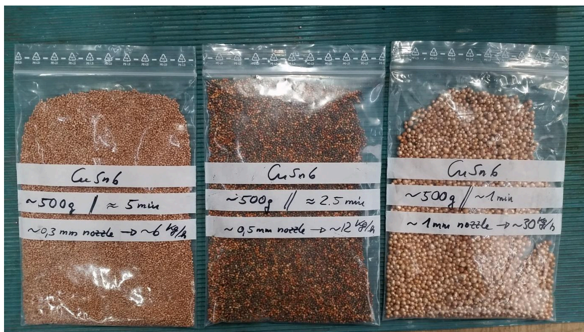
Figure 48: Typical results and process parameters
