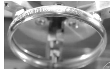
Fig. 5-4 – Example of product with engraved curved or circular surface (with self-centring spindle accessory)
