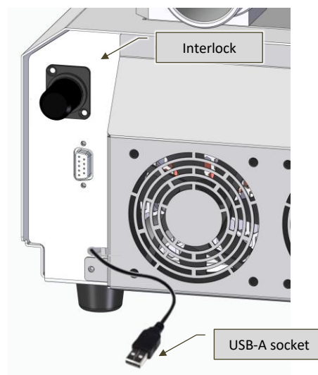
Fig. 6-16 Location of further machine connection points – left rear side view
