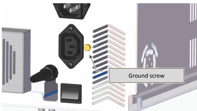
Fig. 6-15 - Location of further machine connection points – right rear side view
