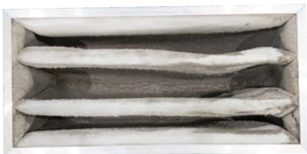
The filter that needs to be replaced
