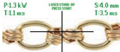
Fig. 7-40 – Example of operational settings display through the vision system
