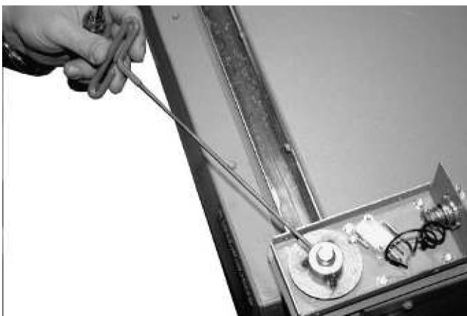
There are several lid and door switch designs in addition to the ones shown here. The top photo shows a kiln lid switch; the bottom one shows a kiln door switch.
